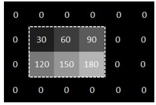
The block or object serializes the image from left to right, one line at a time. The timing diagram shows the control signals and pixel data that correspond to this image. The diagram shows the serial output of the Frame To Pixels block for this frame.
