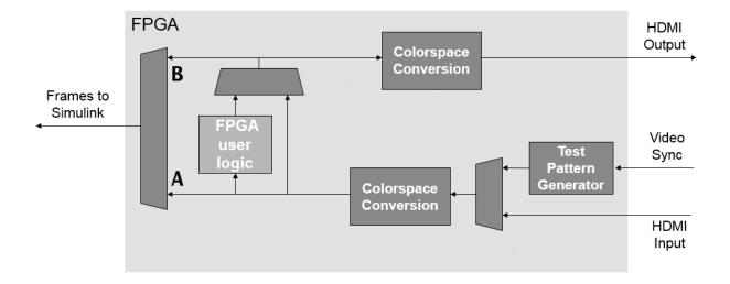
**Note** The reference design on the Zynq device requires the same video resolution and color format for the entire data path. The resolution you select must match that of your camera input. The design you target to the user logic section of the FPGA must not modify the frame size or color space of the video stream.
