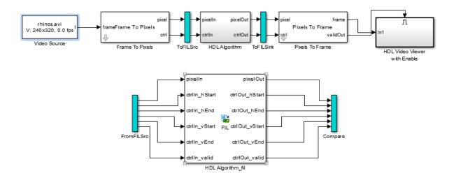
The blue ToFILSrc subsystem branches the pixel-stream input of the HDL Algorithm block to the FromFILSrc subsystem. The blue ToFILSink subsystem branches the pixel-stream output of the HDL Algorithm block into the Compare subsystem, where it is compared with the output of the HDL Algorithm\_fil block. For image and video processing, this setup is slow because the model sends only a single pixel, and its associated control signals, in each packet to and from the FPGA board.
